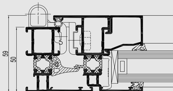
CS 59 is a thermally improved three-chamber system for windows and doors. The system is available in a variety of aesthetic shapes to match the current architectural styles whilst offering all types of both inward and outward opening windows and doors.
