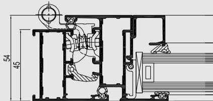
The ES 45Pa is a inward and outward opening system designed according to European standards offering superior quality. Because of 3 layers of gaskets the performance is guaranteed in every situation.
